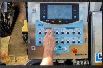
The superstructure can be controlled with the controlling panel with 9" colour intuitive display or radio remote control AUTEC.
