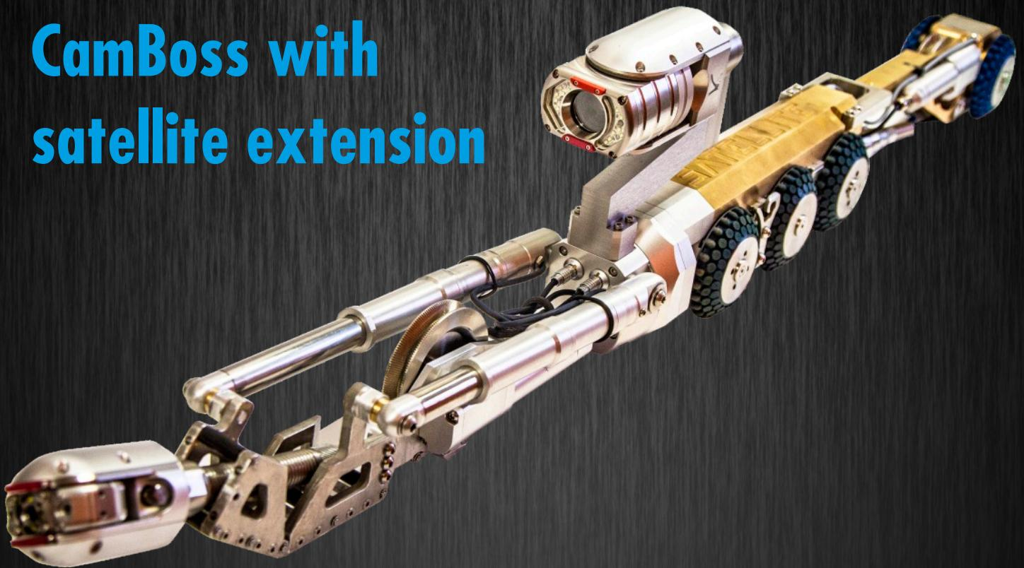
Satellite extension of the crawler Boss 150 (6 x 6) for pipe inspection in DN 150 – 1000. View camera is component of the satellite extension, inspection of pipe connections is enabled by rotary camera head KZ60.
